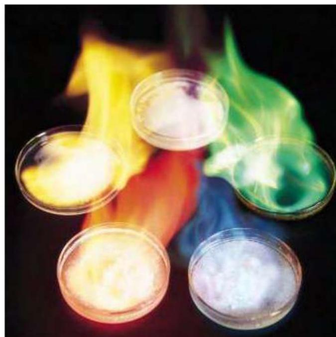
It is an effective and easy experiment that students can easily observe in the laboratory. A perfect display of the visible spectra, this flame experiment reveals the perfect colors of metal ions.- Add a few milliliters of alcohol to a few petri dishes and add a different metallic salt to each dish, and then light the solution and watch it react!
